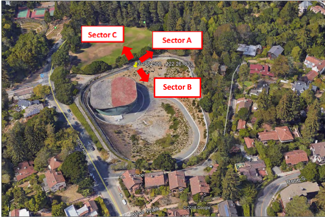
Figure 3: Approximate (i) location of Monopine and (ii) azimuth orientations for the three proposed antenna sectors (Source: Google Maps; Annotated by Dr. Kramer).
